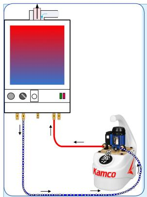
CHOICE OF DESCALING CHEMICAL: The heat exchanger of most combination boilers is stainless steel, and SCALEBREAKER FX OR SR Crystals should be used.
